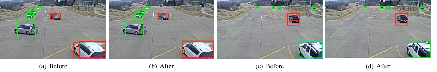
Fig. 10: Effect of result merging. The detection accuracy of the red boxes is improved after applying result merging.
