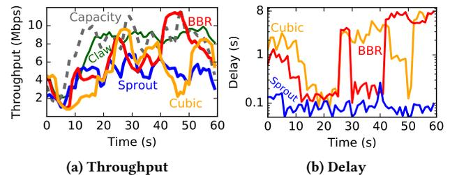
**Figure 1: We use Mahimahi [3] to emulate the cellular network conditions by replaying a Verizon LTE driving trace [5] between a client and server. The client downloads a 100MB file from the server with different CC schemes.**
